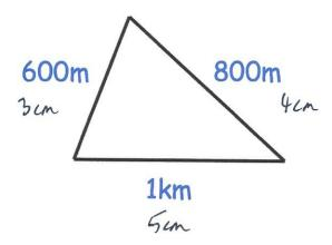
Using the scale of 1cm = 200m, construct a scale drawing of the triangle shown.
