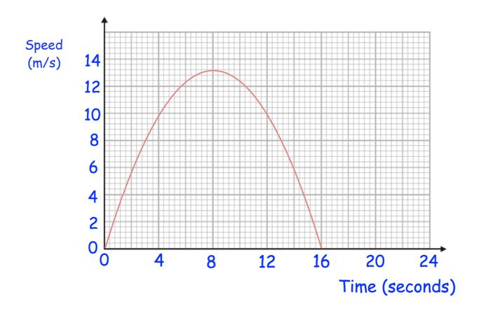
Work out the average rate of acceleration between 0 and 4 seconds.
